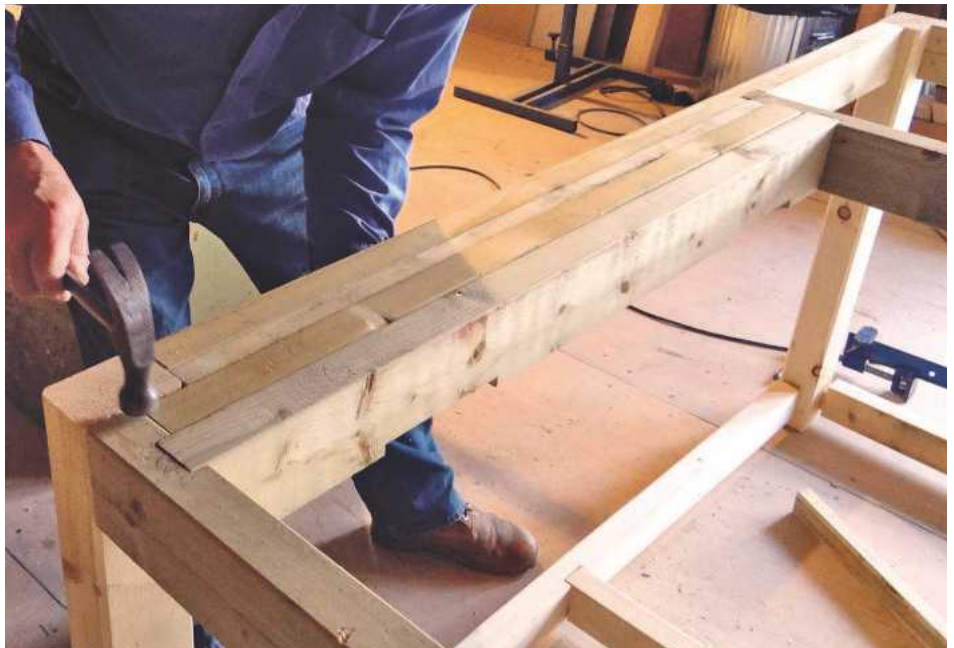
▲ Pic.4 Between the jointed cross rail is a free rail (here being hammered) and some roofing batten to make up the gap. Too many joints would have weakened the very area I was trying to strengthen. These pieces were then cut out for the vices and copiously screwed to each other
